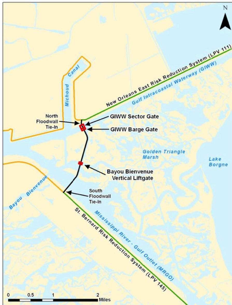
Army Corps of Engineers diagram of the Lake Borgne Surge Barrier's placement.
