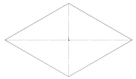
STEP 1, TO FIND CENTER OF MATERIAL CONNECT THE CORNERS. THIS WILL WORK FOR SQUARE OR RECTANGULAR MATERIAL. DRILL 1/8" DIA HOLE AT CENTER. SCREW MATERIAL DOWN TO WORK SURFACE & WITH STRING COMPASS DRAW 20" RADIUS
