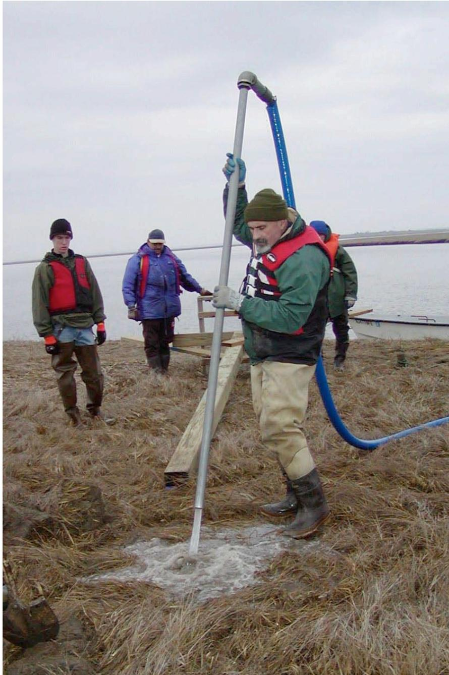
Attached to the pump's hose is a 6' galvanized "L" shaped pipe. One individual will allow the water to do the work.
